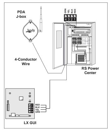
Figure 10. LX Heater Connection to Power Center
